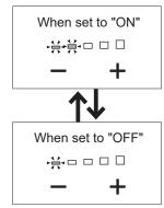
To confirm the option set, check the "Water pressure" LED
