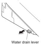
Release your hand to return the water drain lever to its original position.
