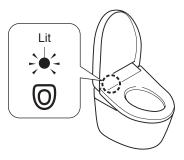
**Note:** If the button is not pressed for about 10 seconds, the "Temperature adjustment" LED will go off, but the setting will be retained.
